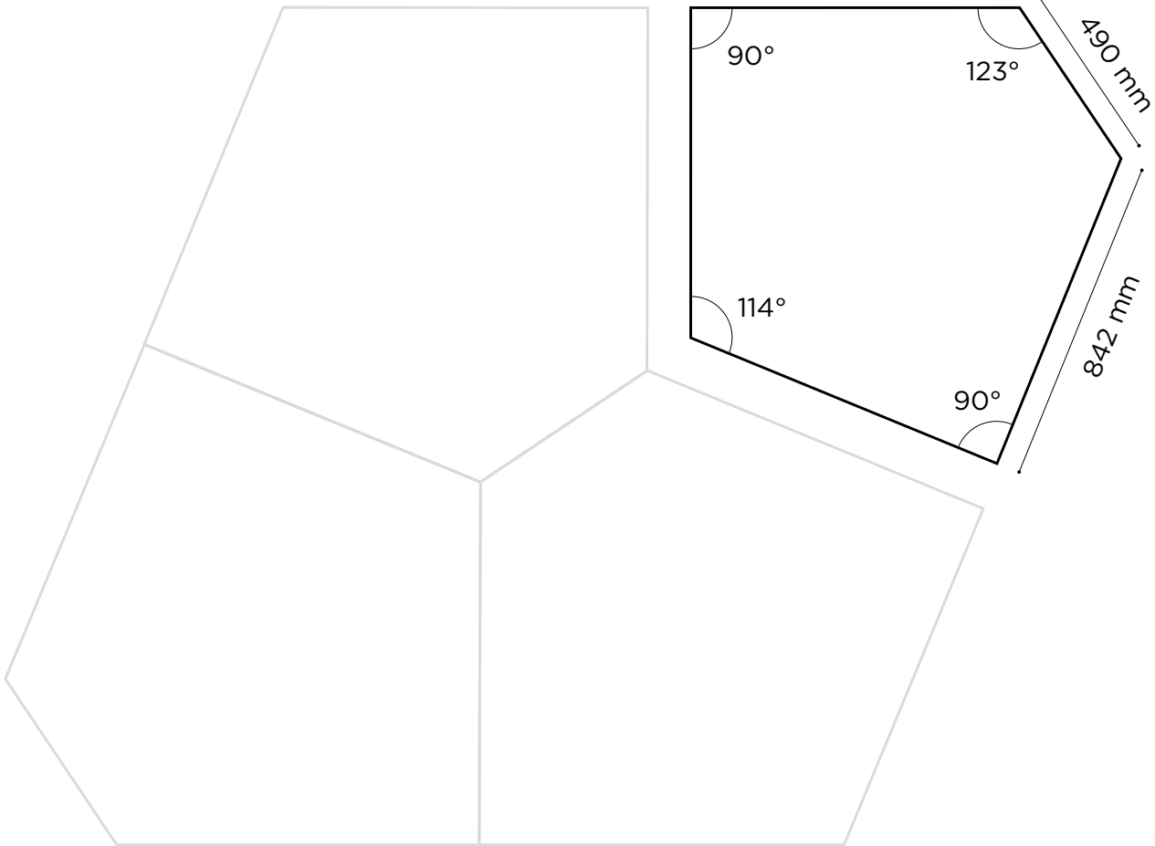
LARGE PENTAGON - MATERIAL \neq 6 mm - QUARTZ \neq 12 mm
